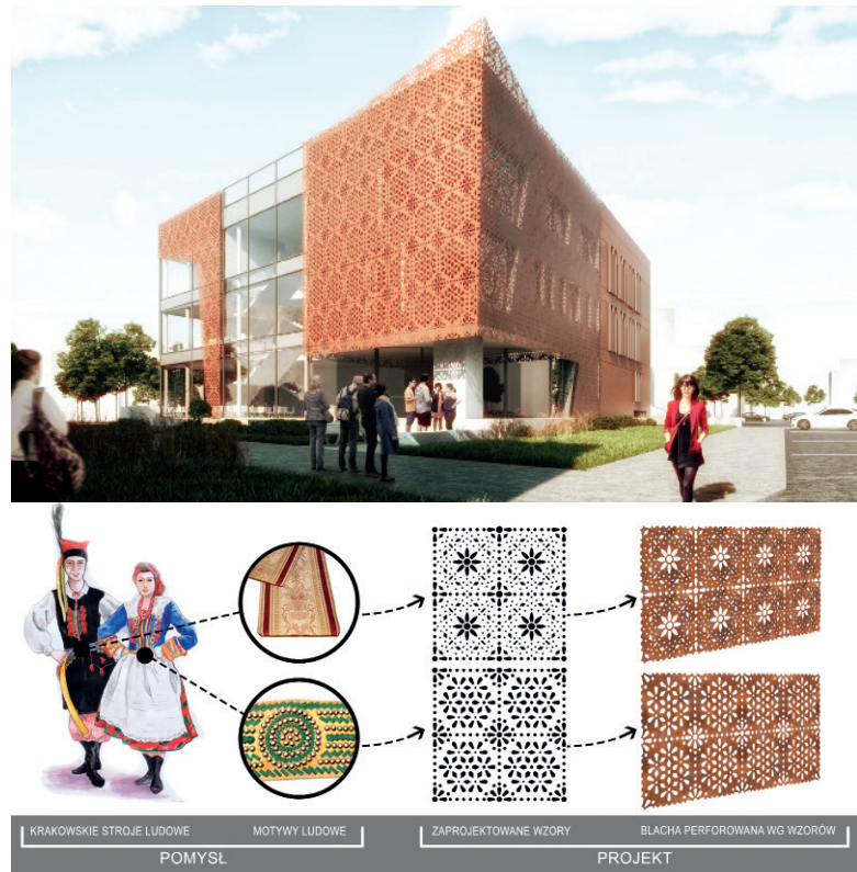
Photo 4. Design of the Ruczaj Centre building, branch of the Podgórze Culture Centre in Kraków (by Studio Budowlane Unity: Janusz Marchwiński, Gerard Jeleń, in collaboration with Michał Dołbniak) - a) front view, b) the authors' motif idea made of corten steel sheet metal (illustration is the author's property; visualisation by M. Dołbiniak)
